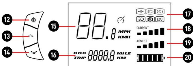
(12). ON/OFF button (13). Change assistance mode and mileage (14). Changing assistance mode and mileage (15). Instantaneous speed (16). ODO: total mileage / TRIP: trip mileage (17). Lights, brake and error indicators (18). Battery power (19). Assistance level (20). Battery level
