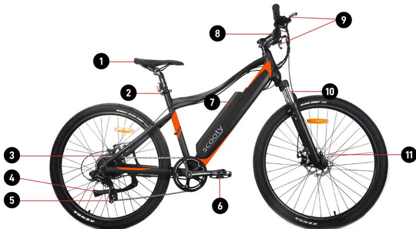
(1). Saddle (2). Saddle adjustment (3). Rear disc brake, motor and gears (4). Crutch (5). Deraileur (6). Pedal (7). Removable battery (8). Screen (9). Brake handles (10). Suspension (11). Front disc brake
